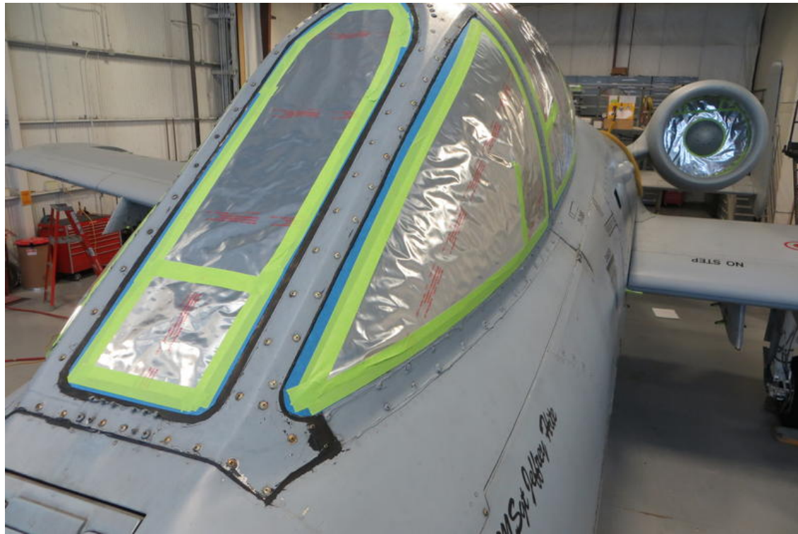
Canopy windows and jet intakes are taped and protected.
